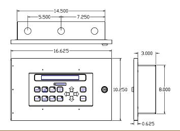
Accommodates flush and surface mounting. 3/4" Conduit Knockouts provided on top of enclosure, hinge on left side. Enclosure may be inverted to hinge on right side, Knockouts on bottom.
